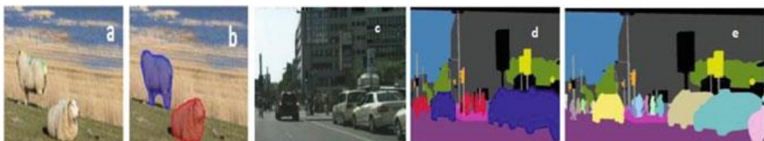
Figure 4. a Image b after applying instance segmentation [113]. c Image d after applying semantic segmentation [114]. e After applying panoptic segmentation [115]
