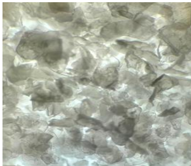
Figure IV.5 : Microstructure of Chitosan: Optical Microscope Image
