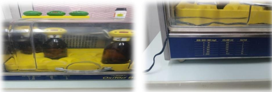
Figure 13: BOD incubator VWR (Personal Photography).
