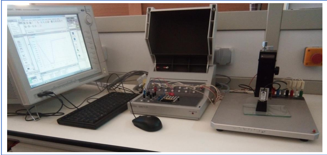
Figure II.25. Real picture of Keithley 2400 type 4 point device .
