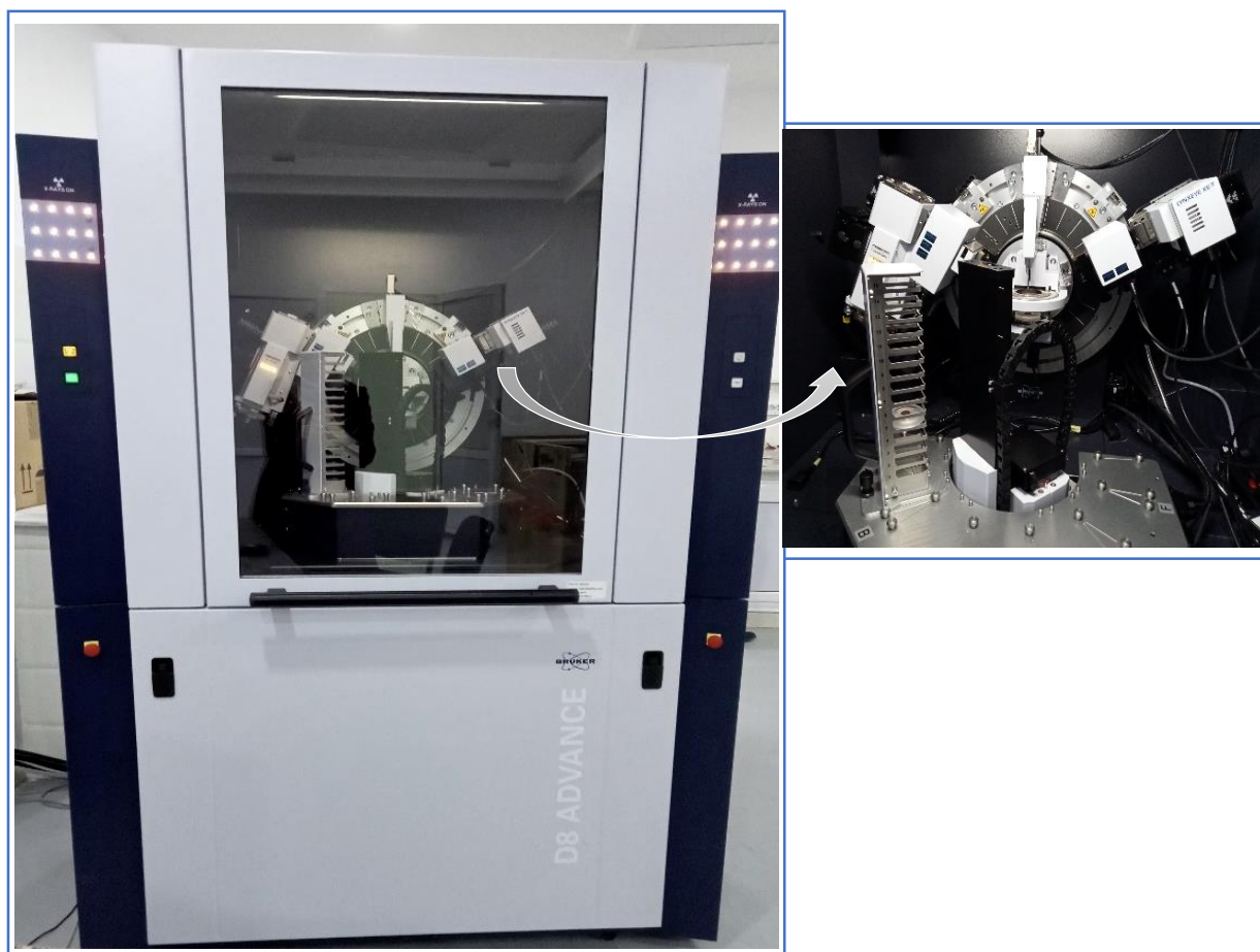
Figure II.16. BRUKER-AXS type D8 ADVANCE diffractometer.
