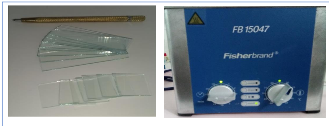
Figure II.7. Cleaning of substrate by ultrasonic bath.
