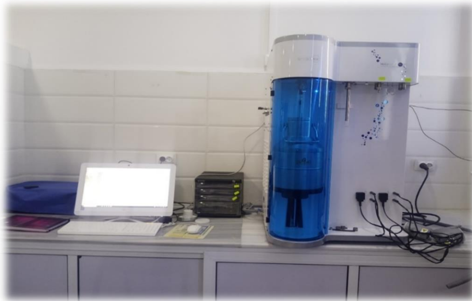
Figure II.10. Nitrogen adsorption apparatus (2017, Quantachrome instruments, version 5.21) (Technology platform for the physicochemical Analysis, CRAPC, University of Constantine, Algeria).
