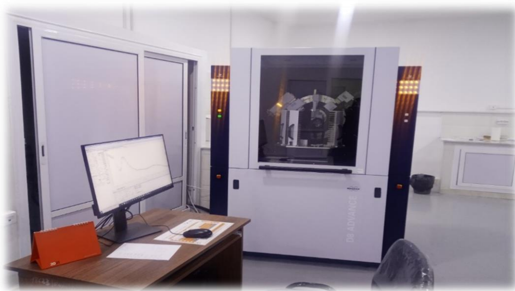
Figure. II.6. Bruker 2D PHASER diffractometer used for XRD measurements (Technology platform for the physicochemical Analysis, CRAPC, University of Constantine, Algeria)
