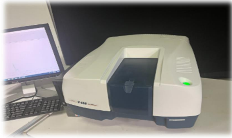
Figure II.12. V-650 UV-VIS Double-Beam Spectrophotometer from Jasco (Technology platform for the physicochemical Analysis, CRAPC, University of USTHB, Algeria)
