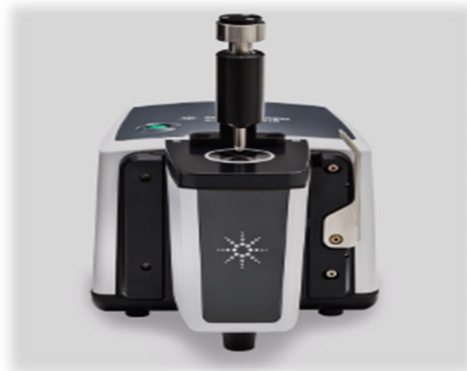
Figure II.8. Spectrometer Agilent for FTIR/ATR analysis, Technology platform for the physicochemical Analysis, CRAPC, University of Biskra, Algeria.
