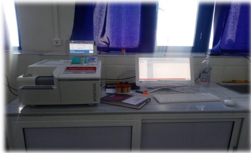
Figure II.11. Differential thermal scanning calorimetric and thermal gravimetric analysis (TG/DSC) apparatus. (Technology platform for the physicochemical Analysis, CRAPC, University of Constantine, Algeria).
