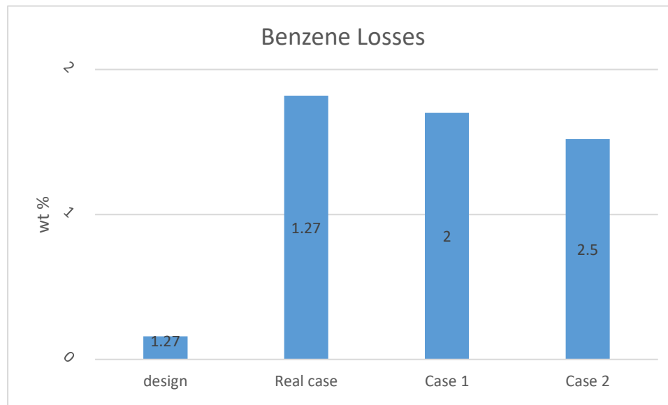
Figure IV.19: The effect of the reboiler pressure on the benzene losses.
