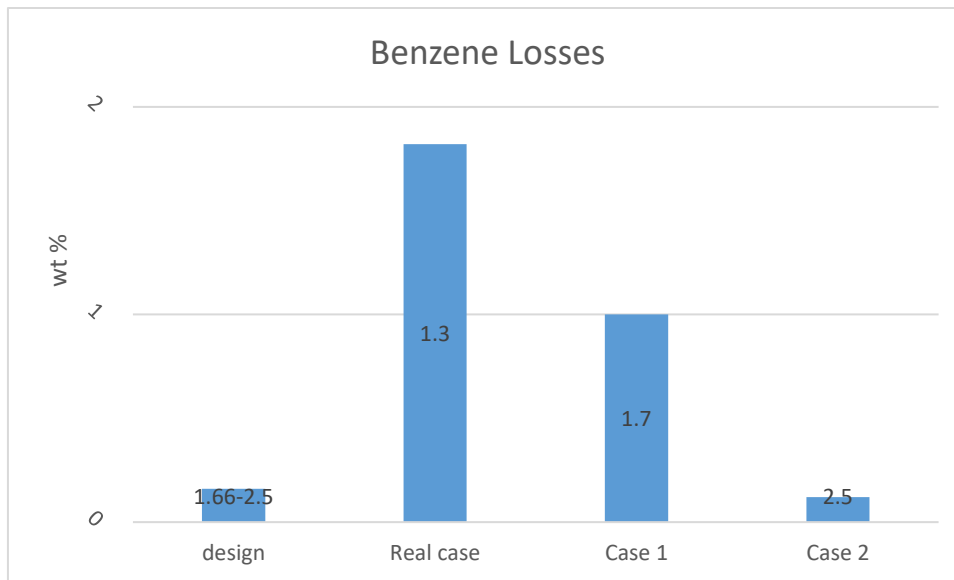
Figure IV.20: The effect of the solvent to feed ratio on the benzene losses.
