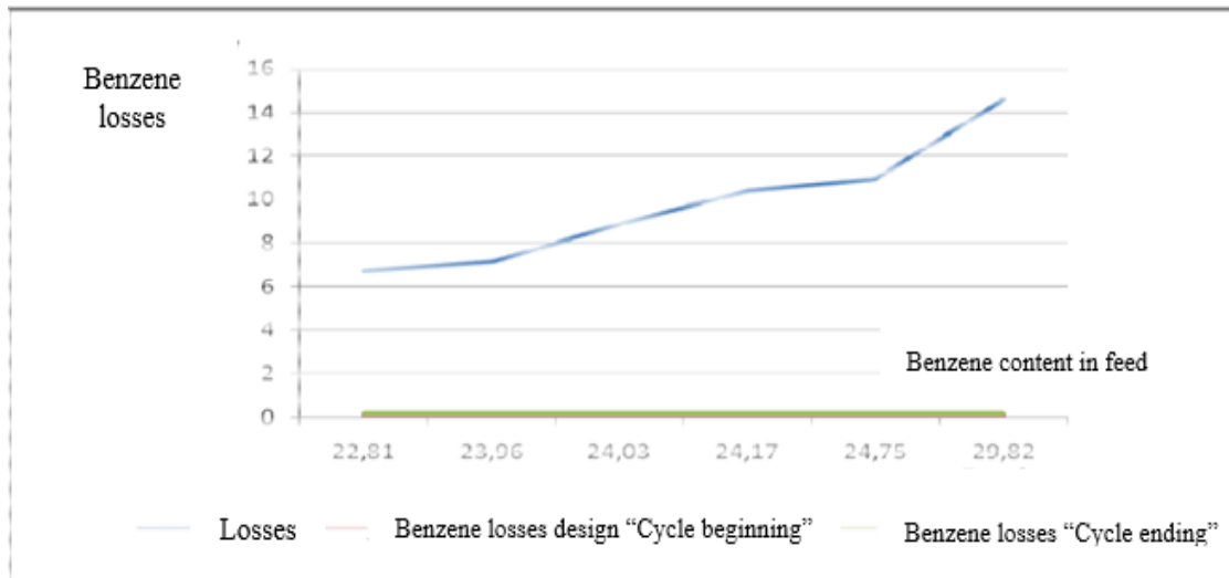
Figure II.4: Losses variation depending on benzene content in feed.
