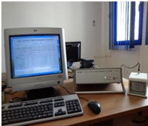
Figure II. 15: Setup of the HMS 3000 Instrument Used for Electrical Characterization.
