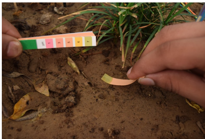
Figure 2.3: Testing Soil pH with pH Papers (STEMpedia 2025)
