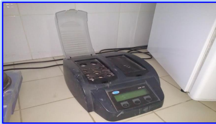
Figure II.20. Photo du bloc chauffant
