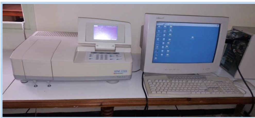
Figure II.11. Image of a Shimadzu 1700 double-beam UV-Vis spectrophotometer.
