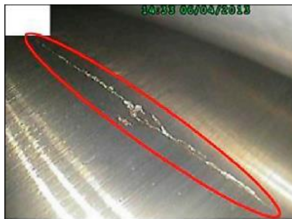
Figure 24 : Inner race fault on the high-speed shaft bearing [99]
