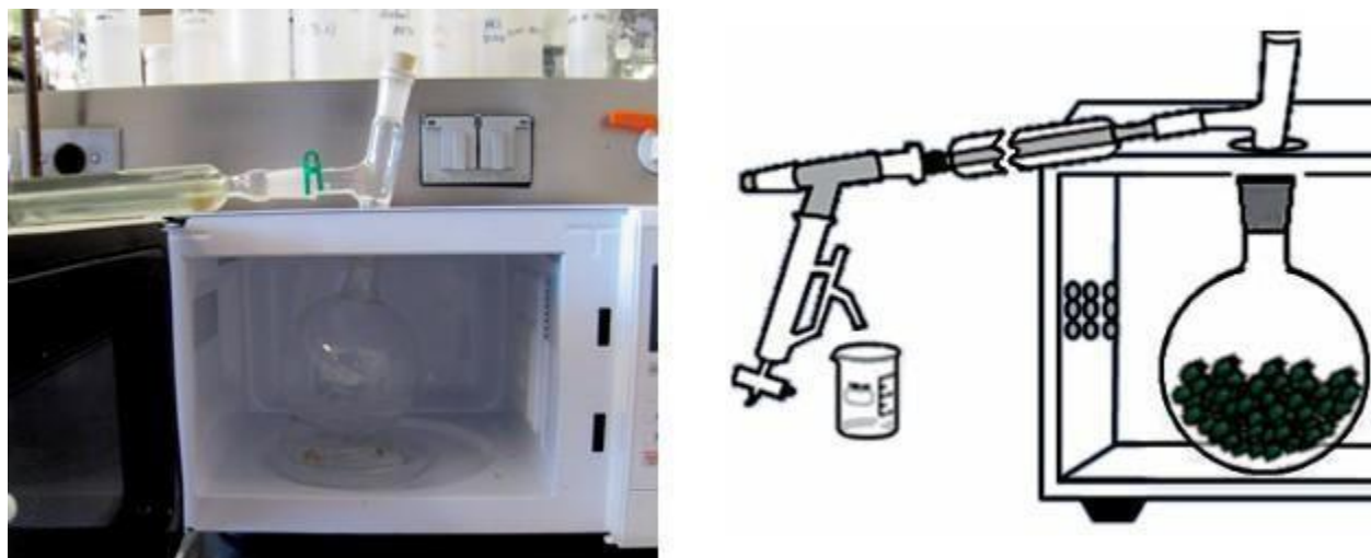
Figure 15: Schematic diagram of the microwave oven adaptation to perform MAE of essential oils from herbs (Cardoso-Ugarte et al. , 2013).
