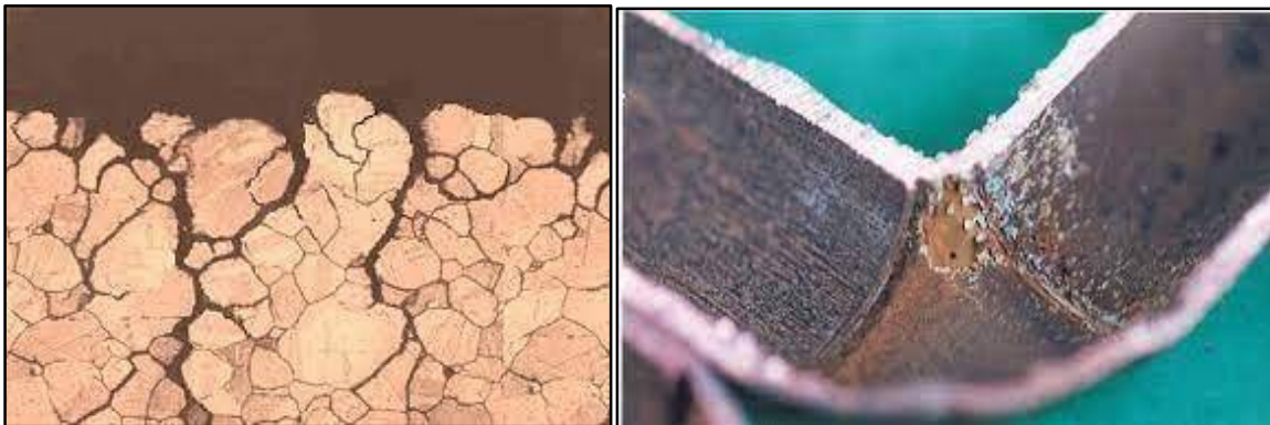
Figure I.9: corrosion sous contraintes.
