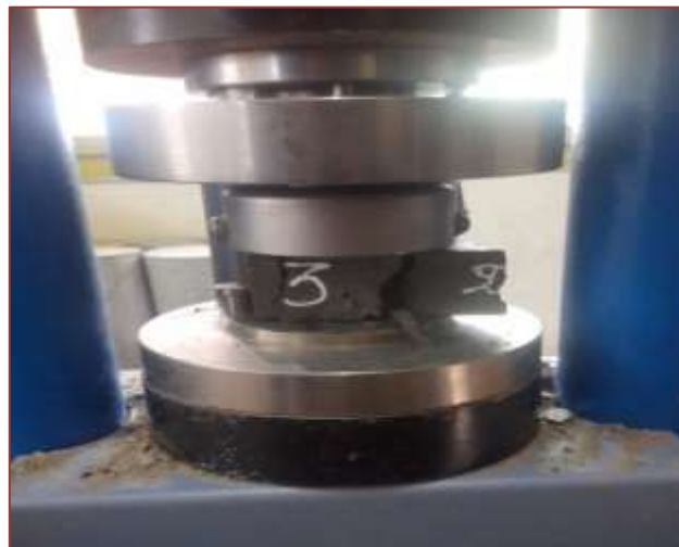
Figure III-16: Essai de compression
