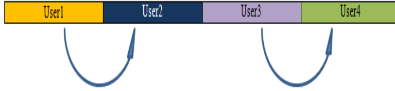
Figure III. 4: Pairing strategies in downlink communication scenario with Near-far pairing (N-F)
