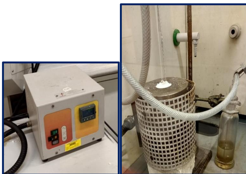
Fig.2.4 Solid-state reaction in small pot furnace.
