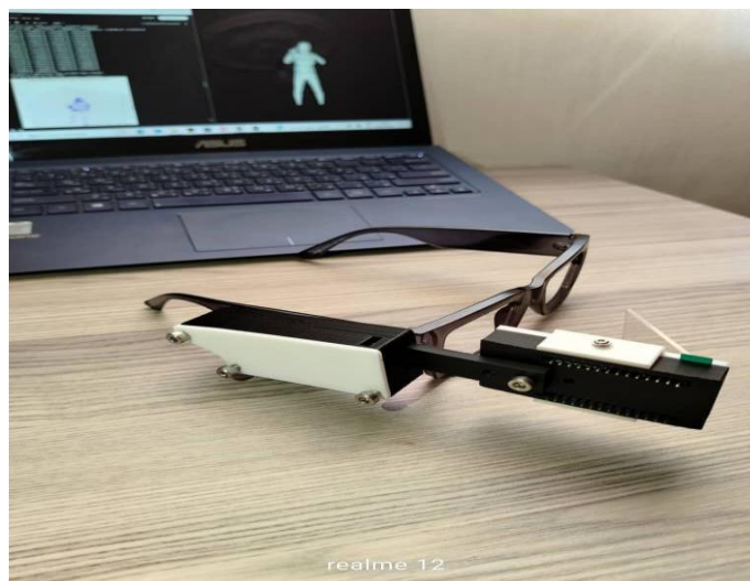
Figure 49: The external face of the first prototype of Smart Sign Bridge
