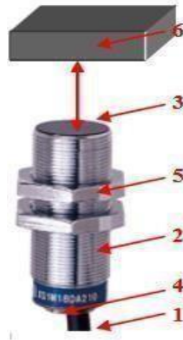
Figure II.8 : External Components of an inductive proximity switch [30].
