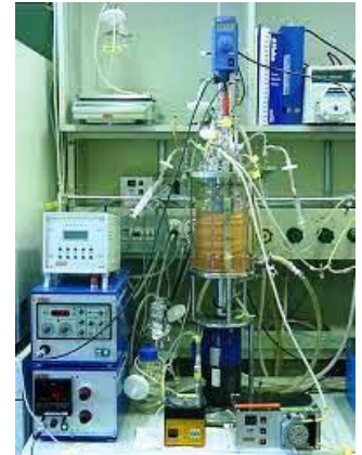
Figure 2: Batch type fermenter (discontinuous) (Carmaux, 2008).
