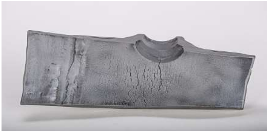
Figure II.8 : Corrosion sous contrainte [51]
