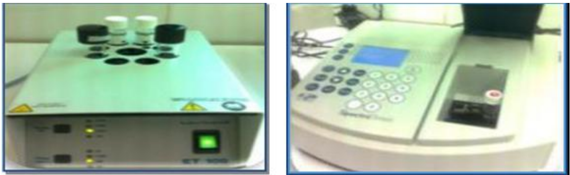
Figure 1.22: Equipment for Measuring Chemical Oxygen Demand: Thermoreactor and Spectrophotometer (Sidi Merouane Wastewater Treatment Plant, 2019)
