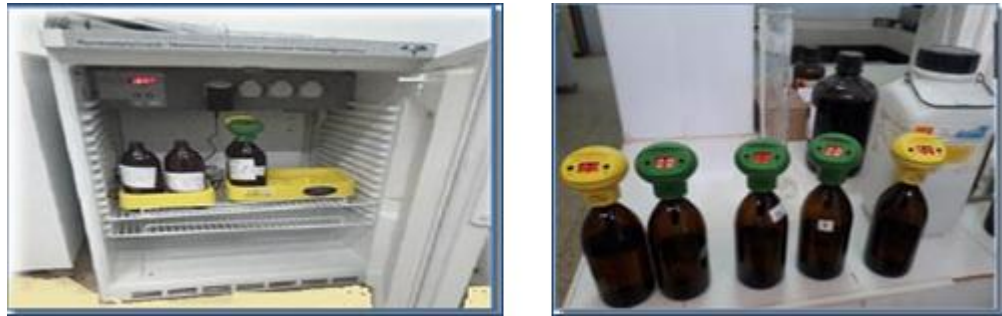
Figure 1.23: BOD Meter and BOD5 Bottle for Measuring Biochemical Oxygen Demand over Five Days (BOD 5 )
