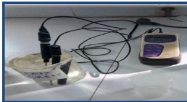
Figure 1.21: Dissolved Oxygen (DO) Measurement by Oximetry (Sidi Merouane Wastewater Treatment Plant, 2019)
