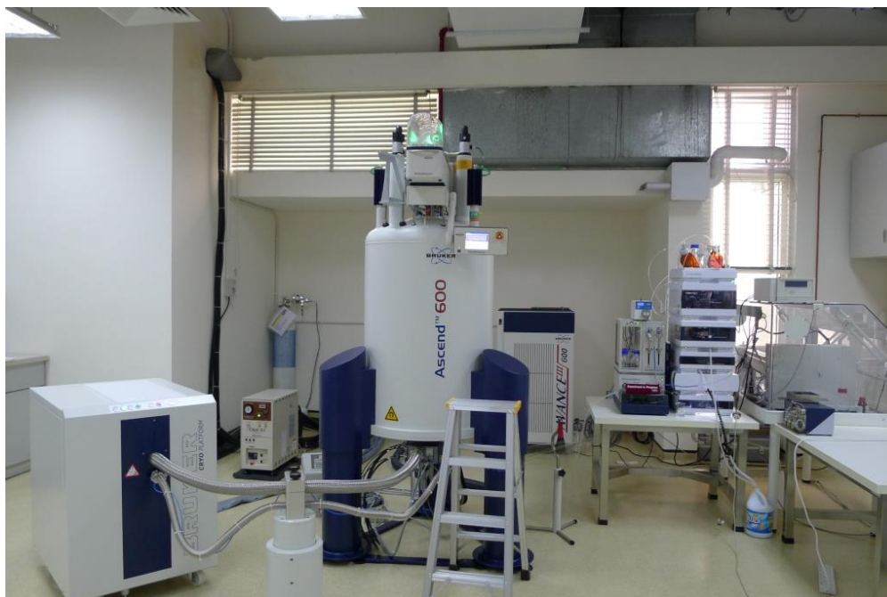
Ultra High Performance Liquid Chromatography (Agilent) – Solid Phase Extraction –CryoFIT Nuclear Magnetic Resonance (Bruker) Analysis.
