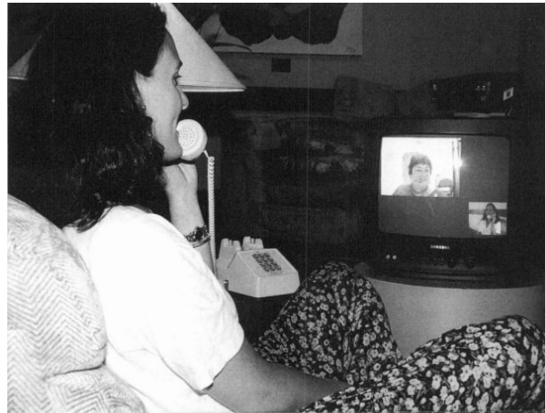
Figure 1.8 : The VC-105 video telephone connected to a standard television and transmitting over POTS. As an option, patient and clinician are able to view both the transmitted and received image, with simultaneous audio. [7].
