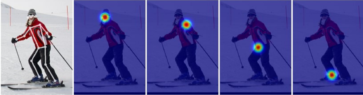
Figure 2.16 : Sample keypoint heatmap predictions made using EvoPose2D, the 2D human pose estimation network [24].
