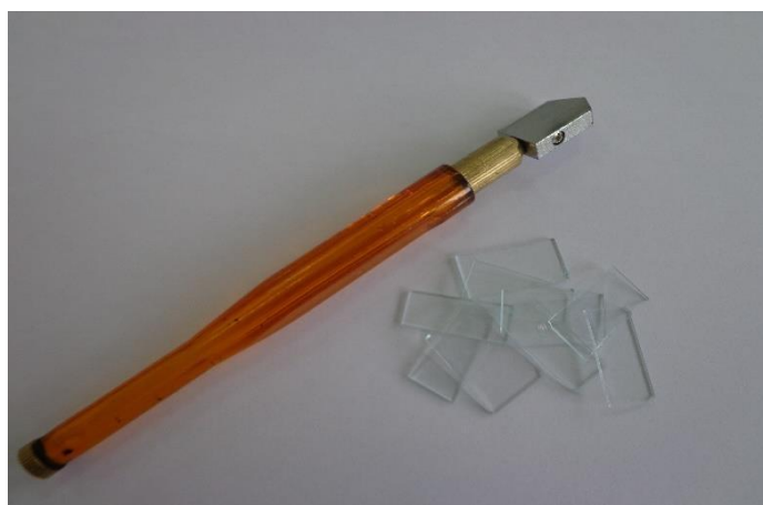
Figure III.1. Isometric glass substrates and diamond pen.
