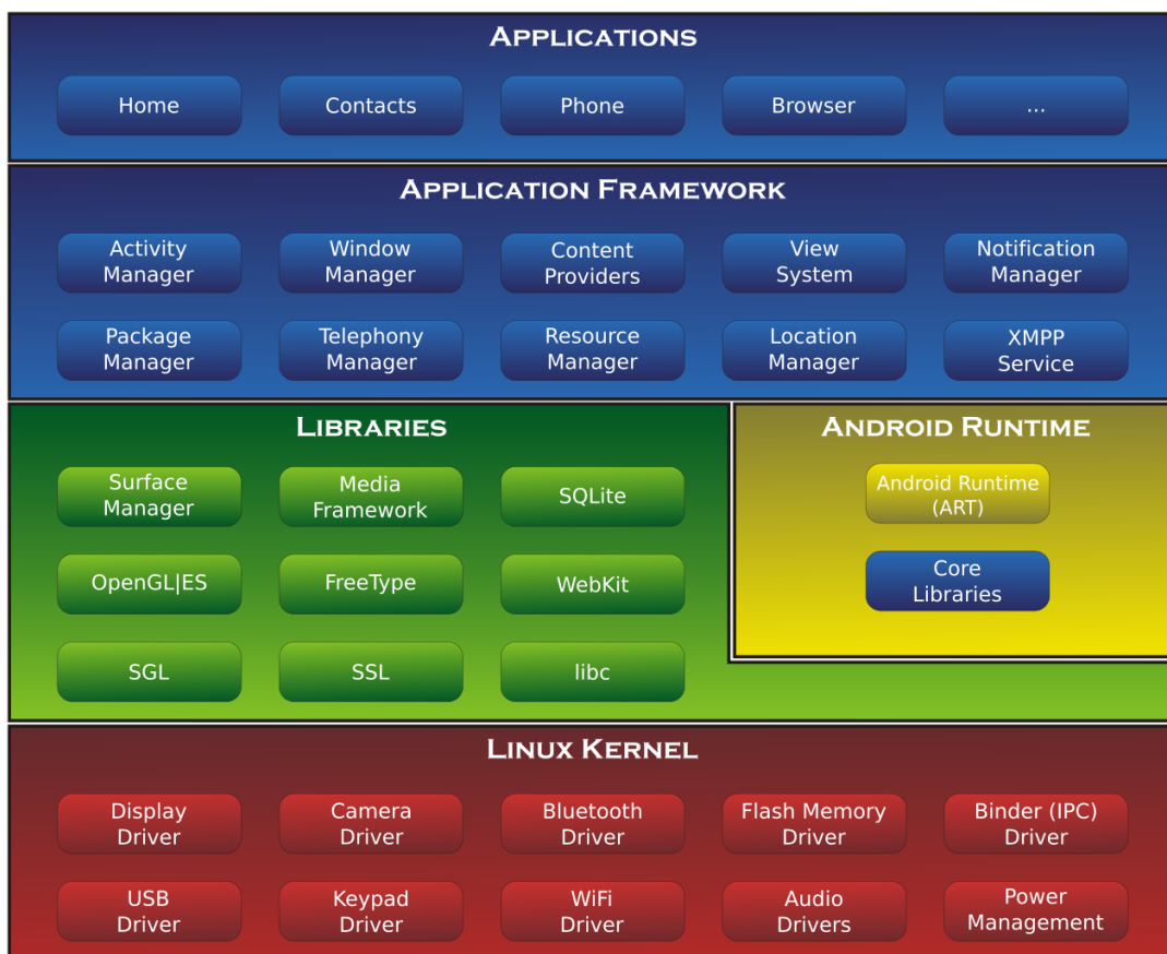
Figure 3.3: Android system architecture layers, from Linux Kernel to Application Framework and user applications. Source: [29].
