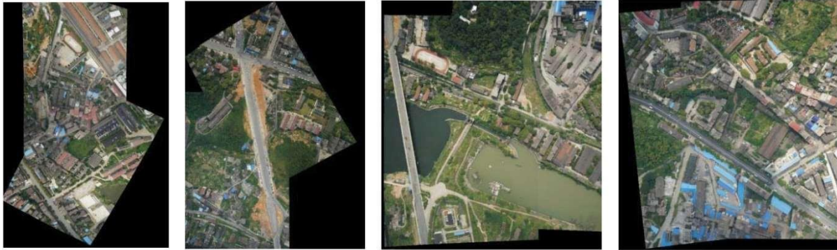
Figure 21: Stitching results of proposed algorithm on aerial sample images.[39]
