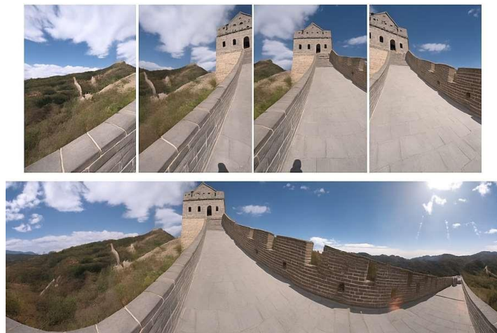
Figure 4: Mosaic stitching technique combining multiple overlapping images without camera rotation to produce a wide field of view composite.[37]
