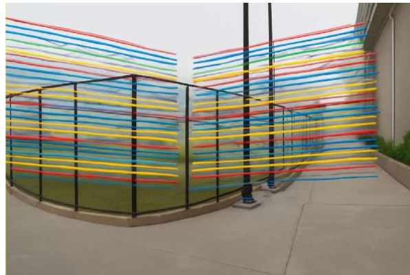
Figure 15: Key point and inlier matching using RANSAC.[19]
