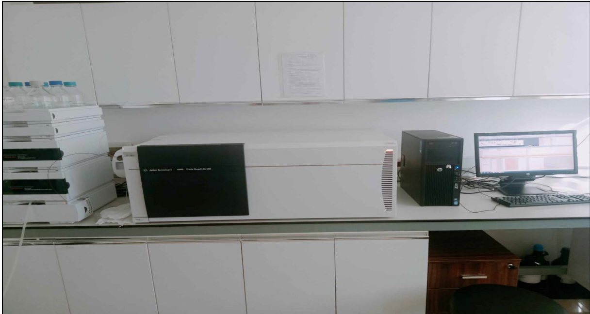
Figure 20: Quantification of polyphenols extracted from the vine wastes using LCMS/MS method (Biorender).
