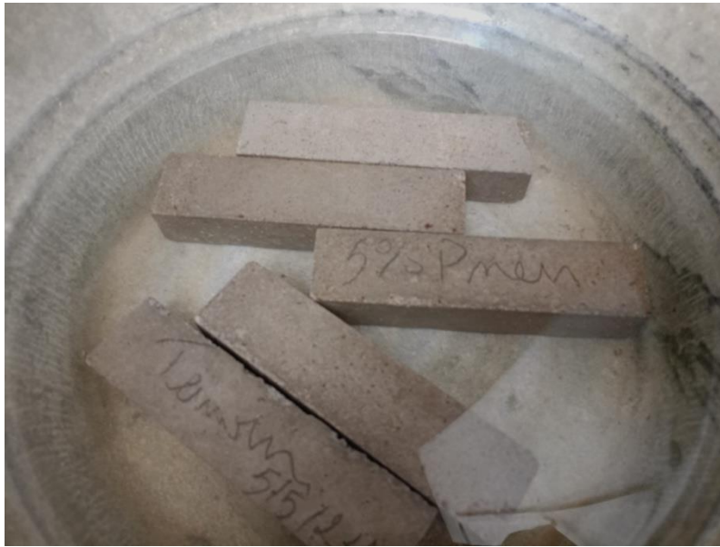
Figure II.7 : Immersion of mortar
