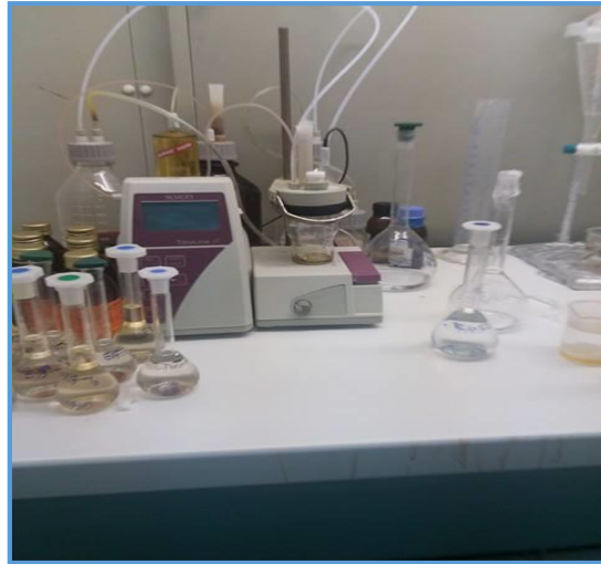
Figure II.4: Karl Fischer Schott Titroline
