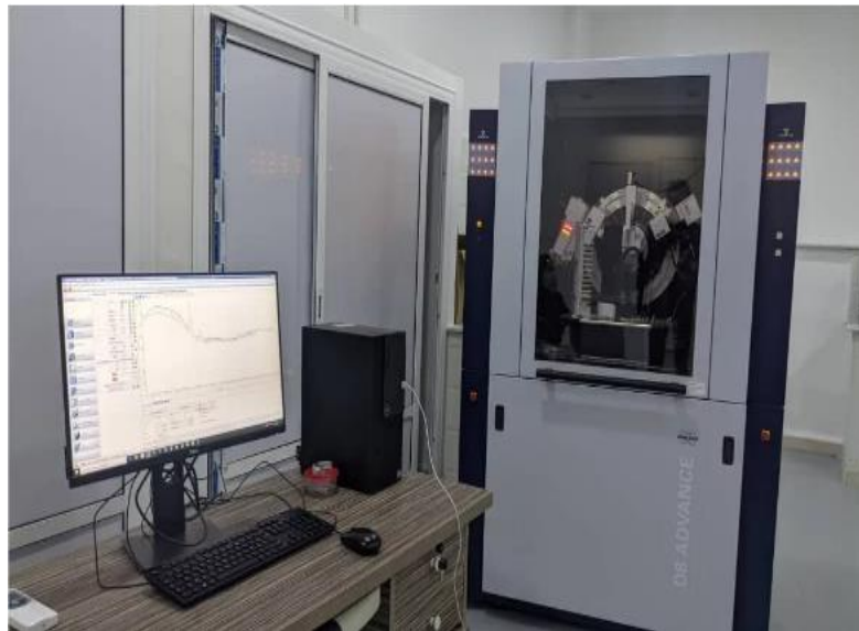
Figure III.11. La diffraction des rayons X (DRX) (Bragg-Brentano).
