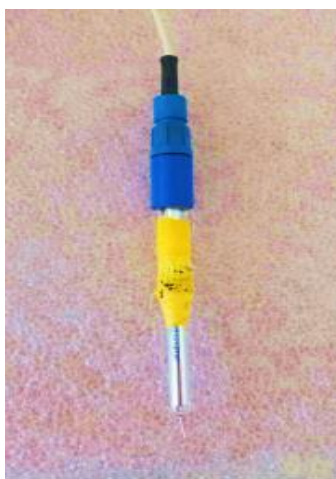
Figure III.7. Electrode auxiliaire de platine [LAIGM] .
