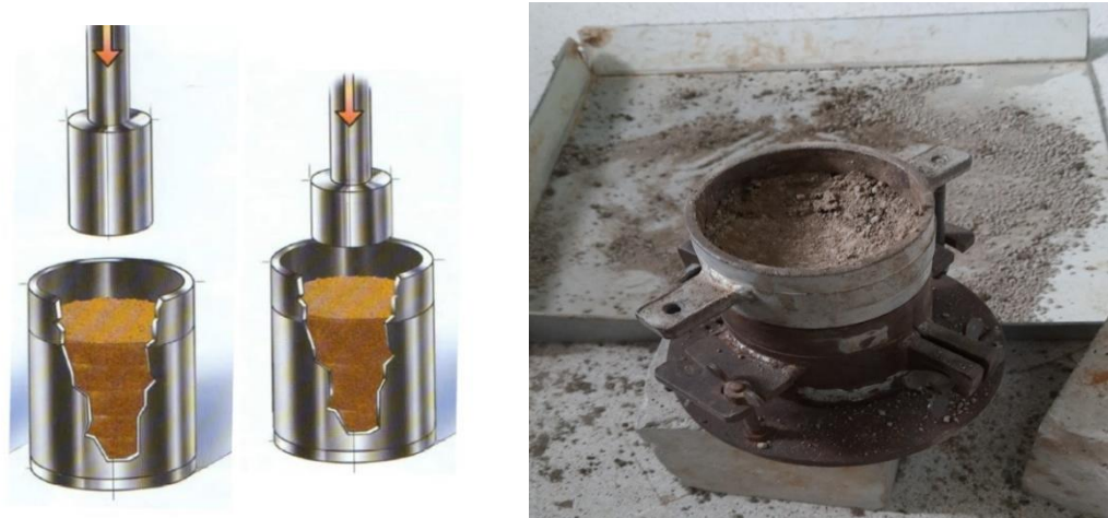
Figure III.6 : Essai de Proctor.
