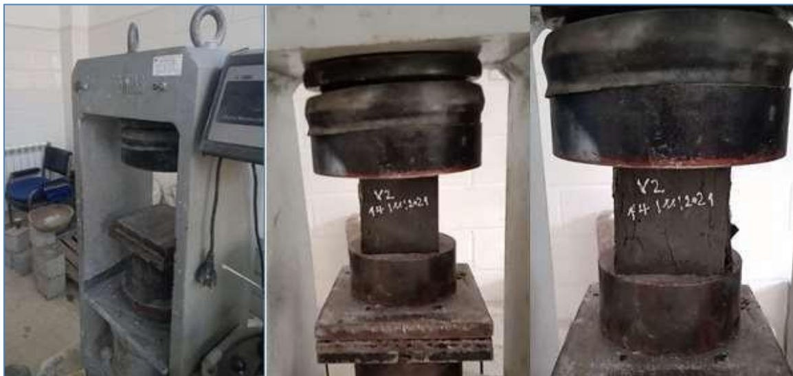
Figure III.10 : Essai de compression
