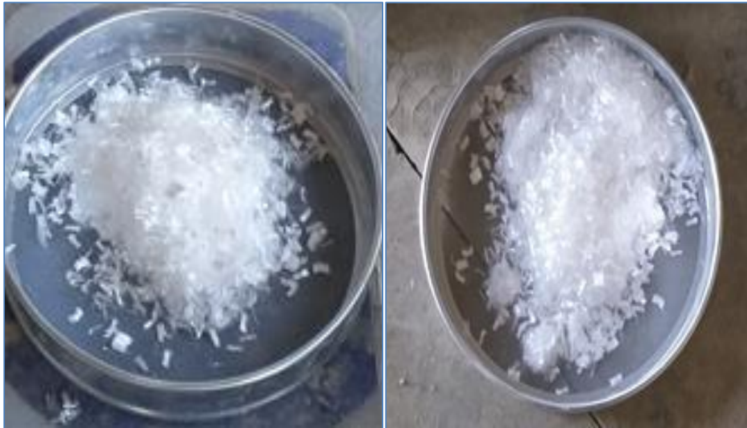
Figure II.11: Fibres de polypropylène
