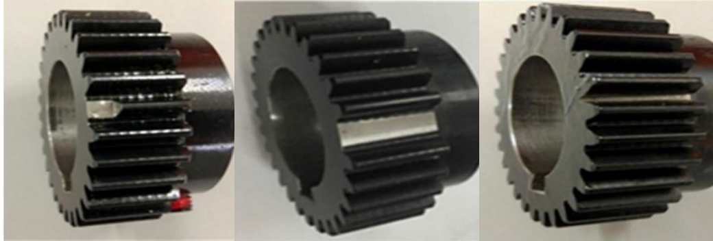
Figure 3.7. (a)Chipped tooth (b)Missing tooth (c)Root crack
