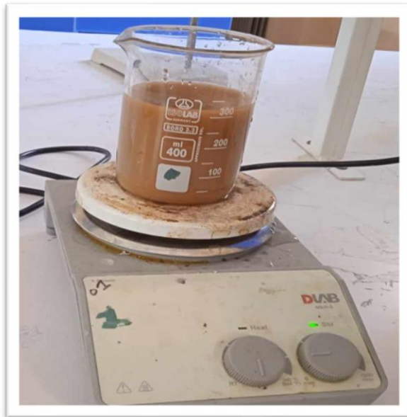
Figure IV.13: Agitation de Zeolite.
