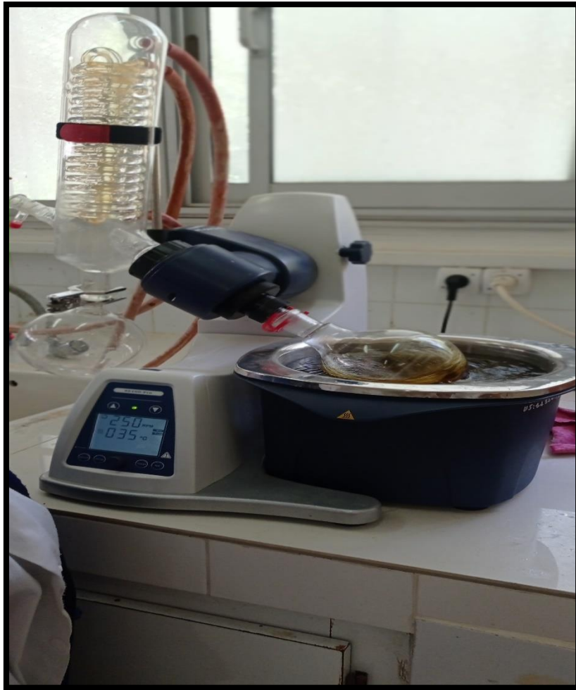
Figure 7: Carob evaporation by BÜCHI rotary evaporator (Original photos 2024).
