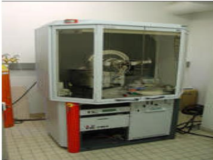
Figure II.4: Diffractometer used for characterization of the deposited thin films.
