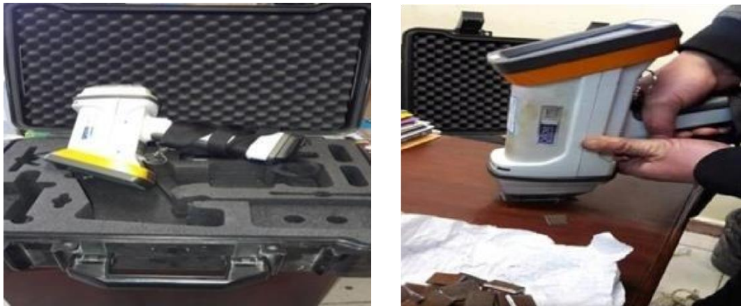
Fig.IV.1 : Oxford instruments X-MET 7000.
