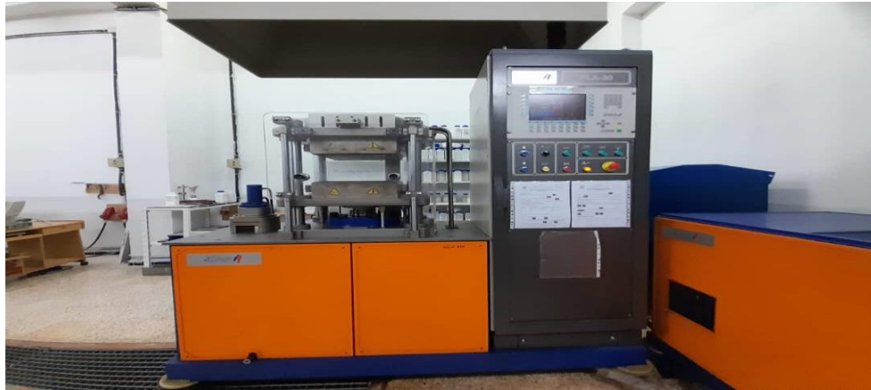
Figure. III.8: Presse hydraulique (ASTM D4703)
