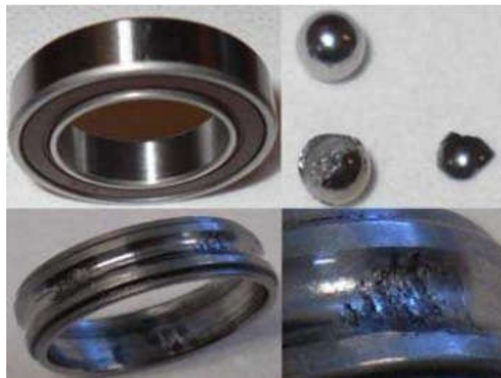
Figure 4-3 Healthy and damage bearings
