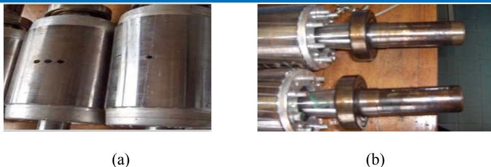
Figure 3-4 (a) 1 Broken bar and 3 Broken rotor bars, (b) Bearing wears
