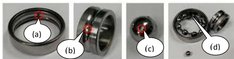
Figure 1-9 Artificial fault related to bearing as: Inner race, Outer race, Ball, and Cage faults [23]
