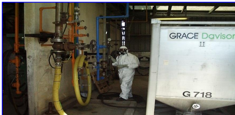
Figure II.10: Catalyst activation step.
