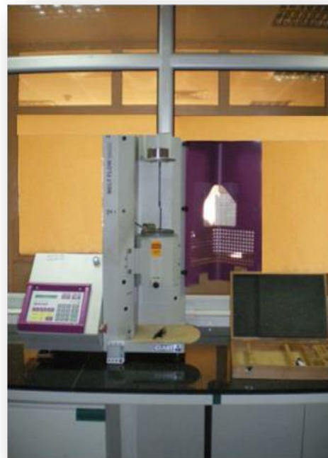
Figure III.1: The Flow Melt Indexer analysis.
