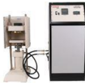
Figure I.22 Curing Chamber HPHT – Model 1910 & Compressive Strength Tester – Model 4207D
