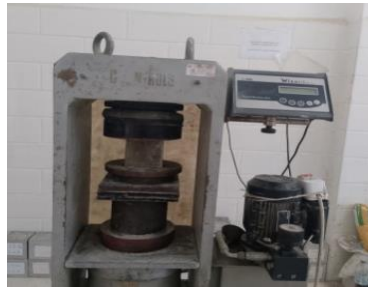
Image 4-7: Essai de compression.
