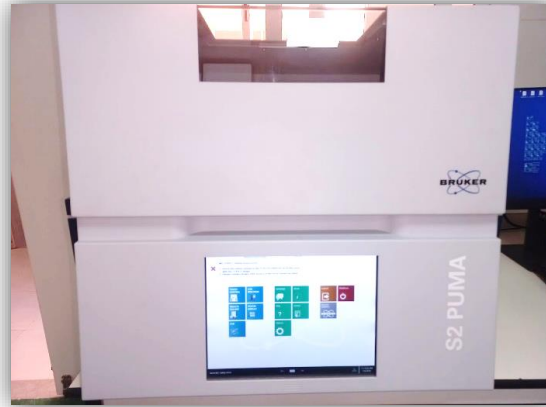
Figure 4 24: Le spectromètre à fluorescence X (S2PUMA-BRUKER) (EDXRF) (XRF).
