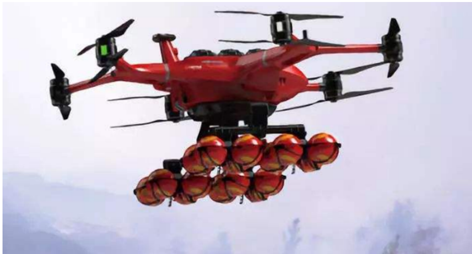
Figure 6.2: Drone equipped with extinguishing balls
