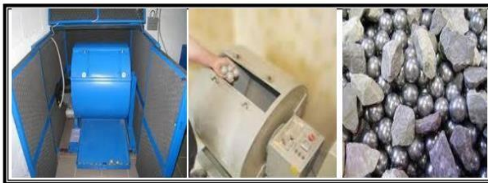
Figure 54 : Essai los Angeles
