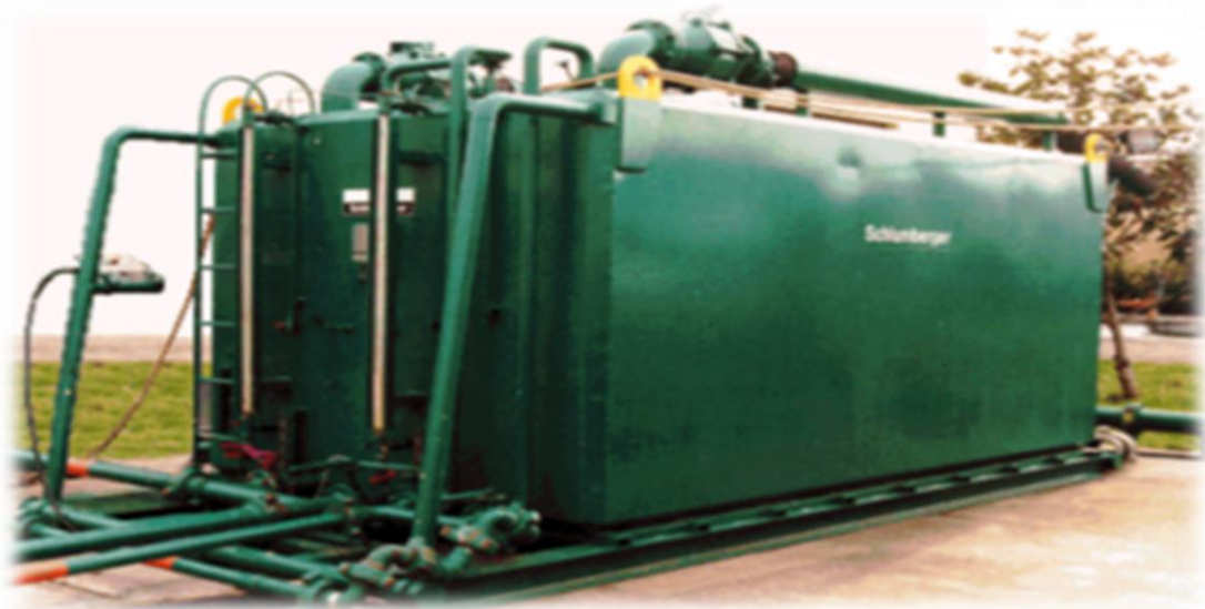
Figure (II-9) : Un surge tank.
