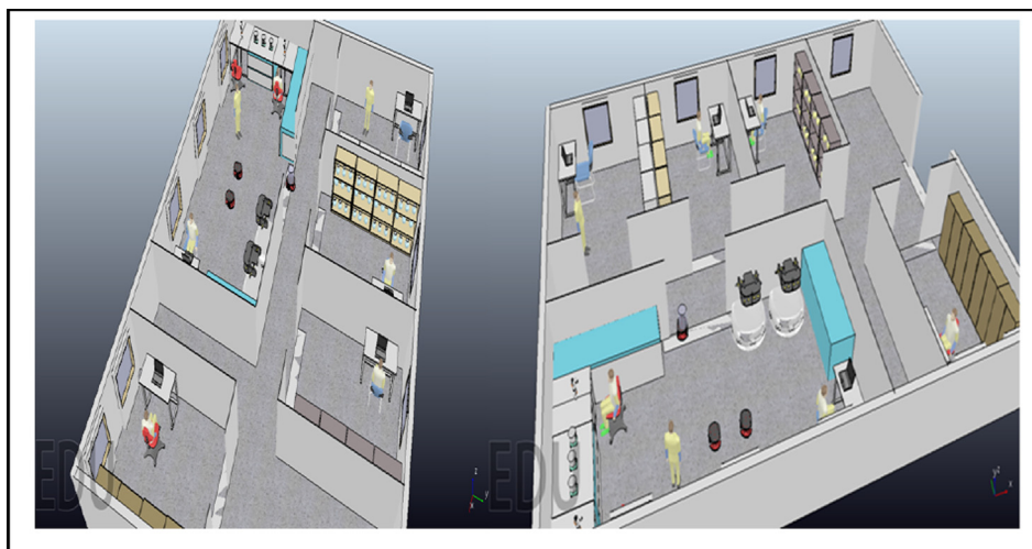
Fig. 8 Representation of a robotic chemical analysis laboratory.
