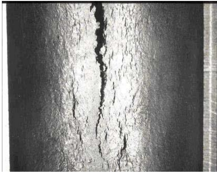
Figure 3.5: Creep rupture of an HK40 heater tube [3].
