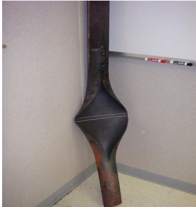
Figure 3. 9: Short-term overheating failure of a vertical, 4.5-in. OD hydrocracker radiant tube [3].
